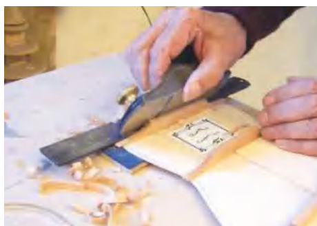
STEP 27. Gabling the back braces
